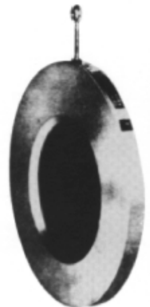
SLIM wafer check valve showing correct position of eyebolt for horizontal installation.
